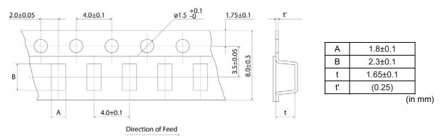
\* The dimensions of the cavity are measured at its bottom.
