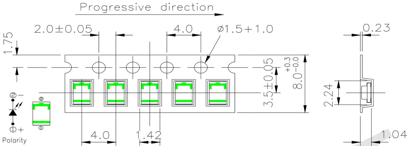
Note: The tolerances unless mentioned is  $\pm 0.1\text{mm}$ , Unit = mm
